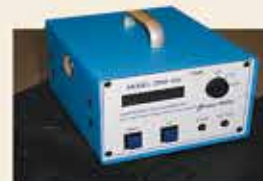
Continuous Radon Monitor (CRM)
